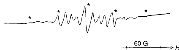
Fig. 3 ESR spectrum recorded following warming of the sample from Fig. 1 to 295 K. (*) Marks invariant lines.
